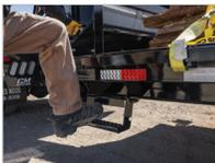
With the retractable monster step, you can step up with the traction step and then move it out of the way when not in use.
