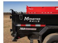
The next generation of PJ dump bodies is capped off by a new rail design that provides strength (2x) than a traditional top rail.
