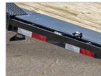
Benefit from enhanced cargo securement with our standard Rubrail, stake pockets and pipe spools. In addition to the built-in stake pockets, the Rubrail provides extra attachment points for securing your load. Customize your trailer further by adding optional D-rings.
