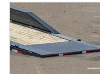
Our 31" Diamond plate knife edge tail makes it super-easy to load low clearance equipment like scissor lifts and fork lifts.
