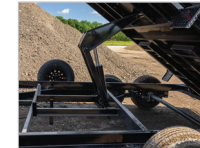
SCISSOR LIFT WITH CYLINDER
