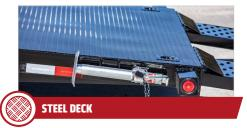
The CH's 11-gauge steel deck provides a highly durable, fluid-resistant floor and includes D-rings and stake pockets to secure your load.
