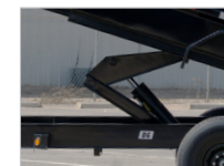
SCISSOR LIFT WITH POWERFUL CYLINDER
